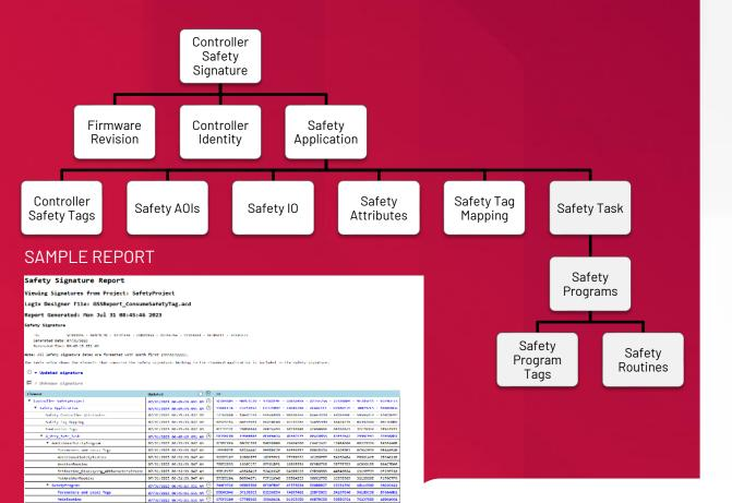
The Granularity Safety Task Signature's concept has the controller compute and verify signatures for every Safety Application Element and rolls them up until the entire Safety Application is accounted for with an overall Safety Signature.
